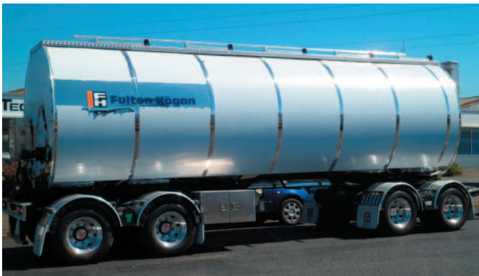
HERA member Transtech Dynamics built this lightweight bitumen tanker for client and HERA member Fulton Hogan
