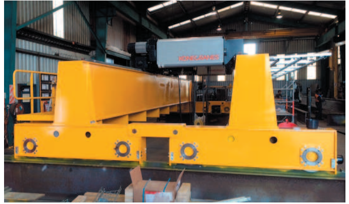
HERA member United Engineering fabricated and installed the components for this 80-tonne crane and structure for client VIP Plastics East Tamaki
