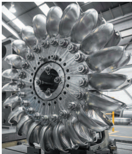
Pelton Turbine Runner for a 3.4MW Hydro scheme to be installed in central Otago designed and built entirely in Christchurch with all the machining completed by HERA member Hydroworks
